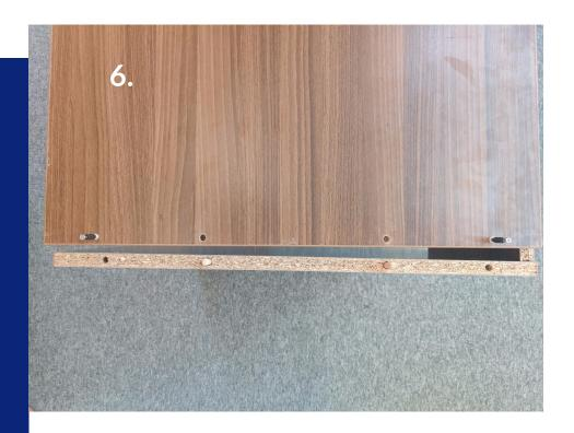
Align the Minifix and wooden pegs of the tabletop and legs and
