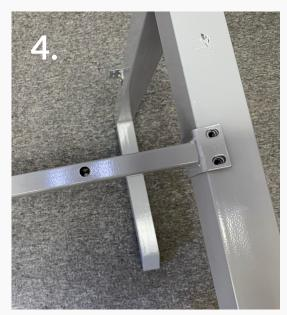
**5.** Use the 8 bronze screws to fix the beam and the legs together.
