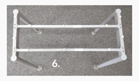
Insert the white bushes into the 3 holes on each beam and 2 holes on each leg as shown with the narrow tip of the bushes going into the hole..
